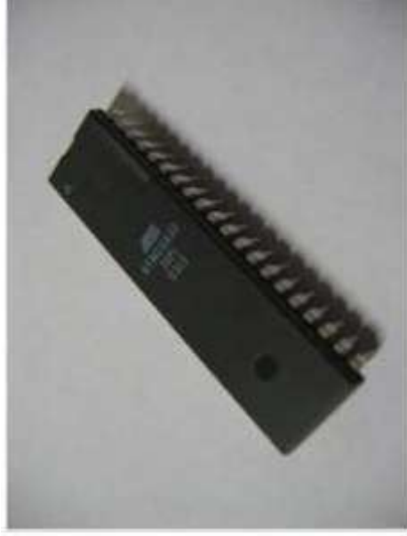
40 pin DIP Photograph of ATmega32
